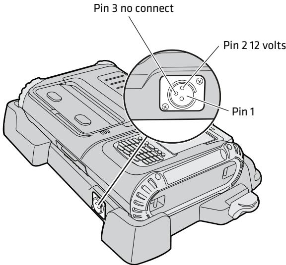
*This illustration describes the pinouts for the vehicle mount power connector.*
